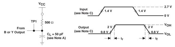
**VOLTAGE WAVEFORMS MEASURED AT TP1, B SIDE**
